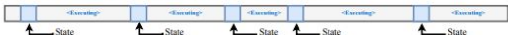
(b) An asynchronous approach to frame skipping. In environments where actions are long or have variable length, the state transition occurs asynchronously. The transition ends once the immediate effects of the associated action have ceased.
